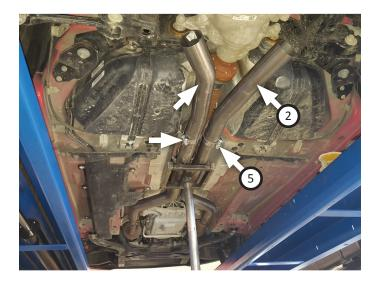
Place clamps (x2) (5) onto left and right muffler assemblies (3, 4) and connect them to mid pipes. Rebolt hanger mounts (x4) onto frame and press hangers into mounts as shown.
