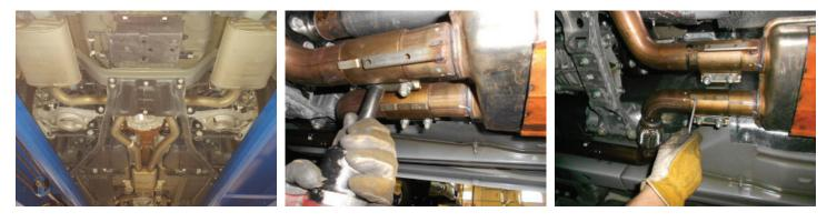
4. Unbolt hangers (x2) behind rear differential. Then carefully slide exhaust system forward and out of rear hanger mounts and lower system to floor. Finally, remove hanger mounts (x2) from rear of vehicle.
