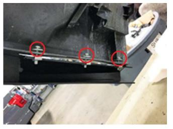
Torque the M4.2 fasteners (both ROUSH-provided fasteners and factory-reinstalled fasteners) to 2 Nm. Torque the fasteners down evenly by first starting at the center and working your way out, alternating from one side to the other.
