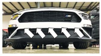
28. Reinstall the front fender liner push pins from Removal steps 2 and 3, less the three (3) push pins that were replaced by the M6 bolts for the canards.
