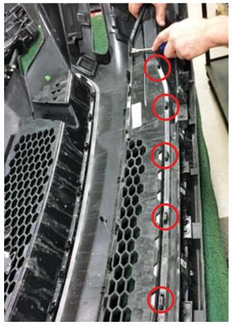
13. Remove the six (6) push pins restraining the end of the OEM chin spoiler to the fascia.
