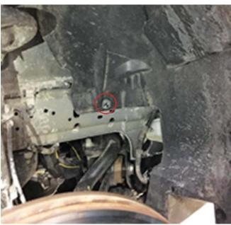
3. Remove the five (5) push pins and remove the fender liner as shown. Repeat on the other side of the vehicle.
