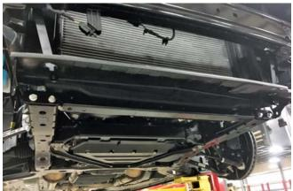
15. Hang the spoiler support bracket (PN: 1318-16F770 for LH and 1318-16F771 for RH) from the pencil braces by hand-starting one (1) M6 fastener through the pencil brace and into the spoiler bracket (PN: W500013). Repeat on the other side. Do not tighten at this time.
