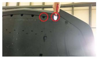
25. Clip two (2) M6 J-clips (PN: N623332) onto the inner fascia and belly pan as shown. Bolt on the canard using two (2) M6x16 (PN: W500013) fasteners and one (1) M5x10 (PN: 11127074) fastener.
