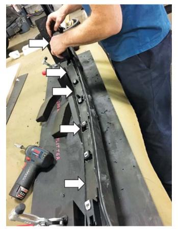
7. Install the chin spoiler onto the OEM fascia by hand-starting the fourteen (14) M4.2 fasteners (eight [8] takeoff fasteners in the center and six [6] [PN: W715060] fasteners at the ends). Note that the tabs on the ROUSH lower grill slide under the upper lip of the chin spoiler. Retain the spoiler by hand. Torque all fasteners to 5 Nm.
