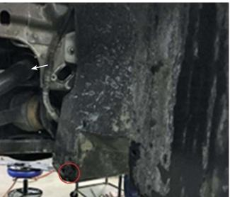
4. Remove the two (2) 8 mm screws from the stone deflector (non-performance package) located on the undertray just in front of each tire.
