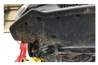
Remove the seventeen (17) (nineteen [19] for the performance package) 8 mm screws from the undertray. Remove the two (2) push pins and remove the undertray from the vehicle. NOTE: Performance package-equipped vehicle shown.
