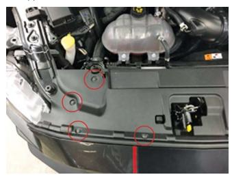
Remove the two (2) 7 mm screws and six (6) 8 mm screws from the upper lip of the fascia. Lift the fascia off the alignment pins and forward off of the vehicle (this step may require the assistance from another person).
