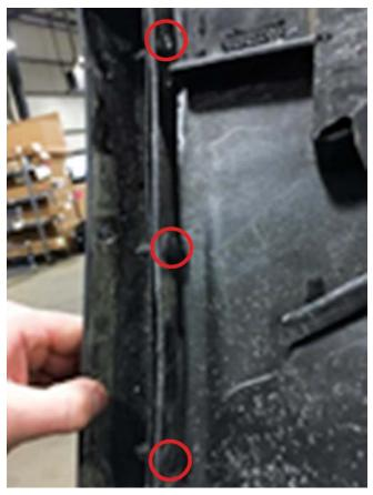
14. Remove the eight (8) 7 mm screws retaining the OEM chin spoiler to the fascia.
