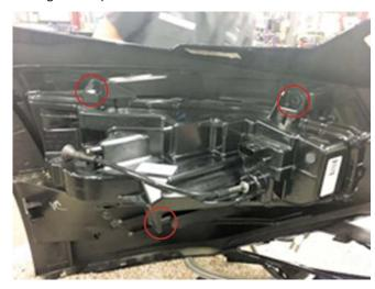
11. Remove the fascia energy absorber structure by prying back the six (6) tabs with a pry tool or trim removal tool.
