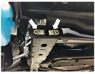
13. Hang the spanner bar (PN: 1318-8K241) by hand starting four (4) M6 bolts (PN: N807309) into the J-clips as shown. Torque to 10 Nm.
