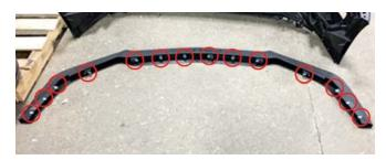
6. Insert the chin spoiler foam inserts (PN: 1318-9U551, 1318-9U552, 1318-9U553, 1318-9U554, 1318-9U555) into the cavities in the spoiler. Start on the LH side, insert 1318-9U551, then move across the chin spoiler, installing the foam inserts in numerical order. NOTE: Insert foam with the arrow on the back of the foam facing up.
