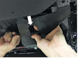
16. Hand-start one (1) M8 fastener (PN: 161821) going through the outer hole of the bracket into the spanner bar as shown. Repeat on the other side of the vehicle. Do not tighten at this time.
