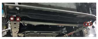
14. Remove only the lower 13 mm nut from the backside of the bumper beam. Slide the pencil brace (PN: 1318-16F774) through the hole in the air deflector and onto the bumper beam bolt and reinstall the 13 mm nut. Repeat on the other side. Do not tighten at this time. **NOTE:** The circular end faces down.
