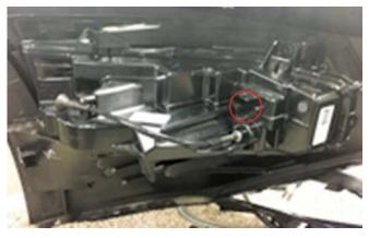
7. Remove the two (2) nuts and one (1) push pin holding the fascia to the fender. Push down on the Christmas tree retaining the bracket to the fender. Repeat on the other side of the vehicle.
