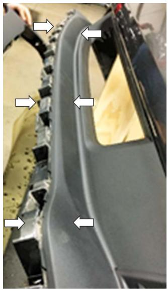
4. Cut out the drill template (PN: 1318-17F775TMPL), check scale with a metric ruler and tape to the underside of the chin spoiler as shown. Be sure to align the template on the **UNDERSIDE** of the spoiler (the ROUSH logo should be facing down). Align the inner edge of the template to the inner edge of the spoiler. Mark and drill the twelve (12) 1/4" holes in the bottom of the spoiler. Trim out the five (5) rectangular sections.
