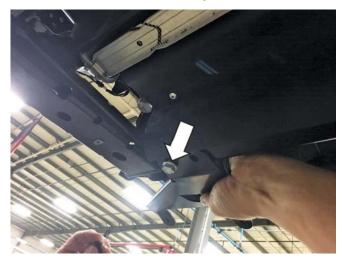
17. Mock install the outer spoiler canard bracket (PN: 1318-6328) by pushing the OEM fascia retainer into the fender and placing the bracket onto the stud. Drill a 1/4" hole in the fender liner by visually lining the drill bit up with the canard bracket. Repeat on the other side of the vehicle. Do not tighten at this time.
