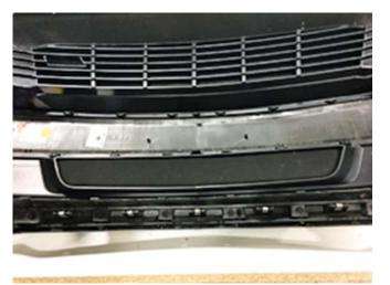
3. Pull the red backing off of the tape on the lower grill and squeeze the lower grill and lower lip of fascia together to wet out the tape. This ensures the tape adheres properly to both parts.
