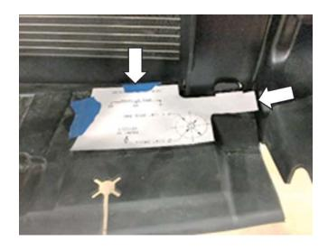
11. Drill a 1/4" pilot hole using the template as a guide. Then drill a 1-1/8" hole with a hole saw using the pilot hole as a guide.
