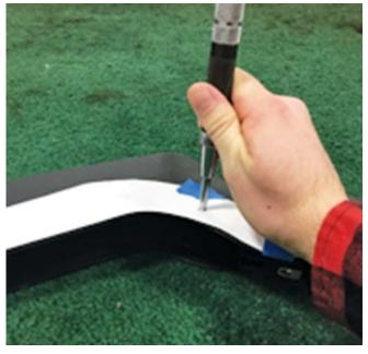
Insert the fourteen (14) M4.2 J-clips (PN: W704823) into the backside of the spoiler, aligning them with their respective holes. Eight (8) clips install into the dog house holes and six (6) clips install into the outboard holes.
